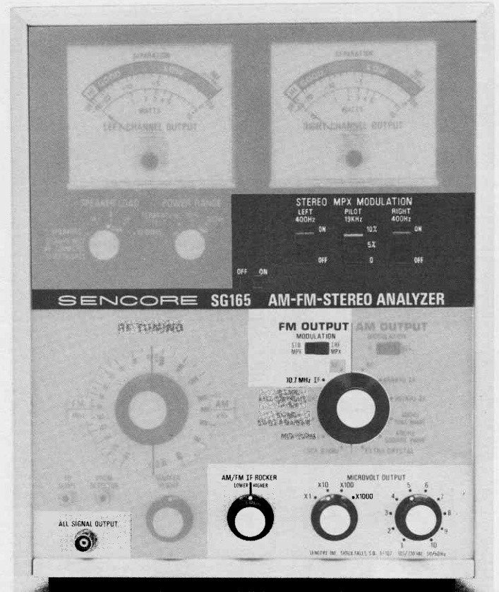
Fig. 14 Operational Controls for 10.7MHz IF
