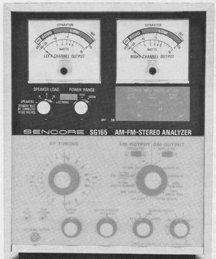
Fig. 11 Output Meters for Power Output Test
